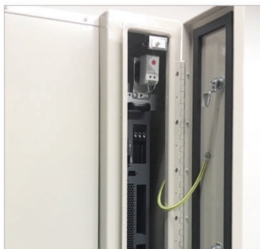
ADLINK Edge & AI Server installed in Charles NEMA 4X (IP65) Enclosure
