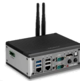
MXE-210 with Intel® Movidius™ Myriad™ X VPU acts as an inference platform to identify the reading. MXE-210 also serves as a gateway, sending the reading to back-end servers for data acquisition and near-real-time monitoring.
