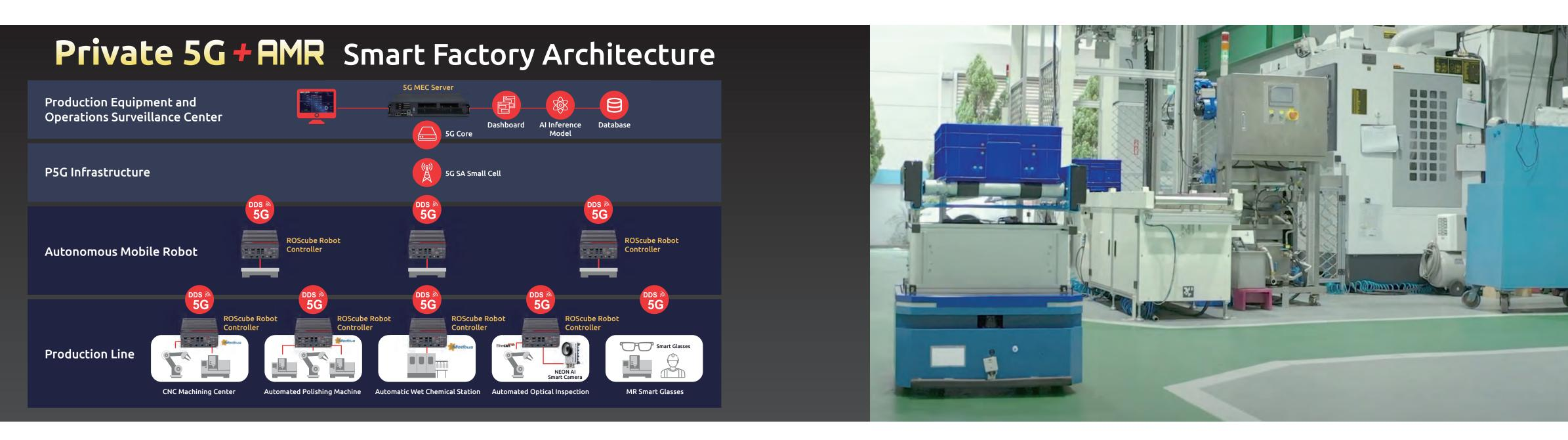
The Production Equipment and Operations Surveillance Center incorporates p5G with DDS to enable real-time integration with production line information and connects with AMR to transport parts and components to various inspection divisions for enhanced productivity.
