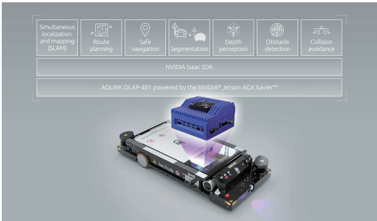
Figure 2. ADLINK DLAP-401 powered by the NVIDIA® Jetson AGX Xavier™ system-on-module delivers very high levels of computing performance for iw.hub.
